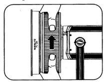
When adjusting the flood light, as shown in the figure, to adjust the beam angle of light, turn the dial on the lens with two fingers, like adjusting zoom on a camera lens to get the flood effect.
