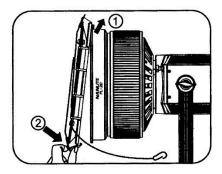
Remove the safety strap in advance, push the the mount of barn door ② while pulling upward the mount of barn door ① and remove the barndoor.
