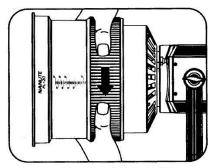
When adjusting the spot light, as shown in the figure, to adjust the beam angle of light, turn the dial on the lens with two fingers, like adjusting zoom on a camera lens to get the focused effect.
