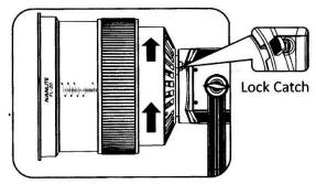
When removing the Fresnel lens, push and hold on the lock catch while rotating the lens and you are able to remove it from fixture.
