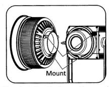
When installing the Fresnel lens, make sure its mount points line up the slots on the light fixture. When the mount points and slot are lined up push the Fresnel lens in place rotate the lens in the locking direction as described on the light.
