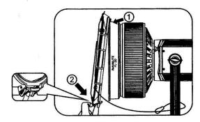
When installing the barn door, make sure the mount points of barn door ① and barn door ② connect properly in place on to this rim of the Fresnel, then connect the safety strap to the light stand. (As described on the light.)
